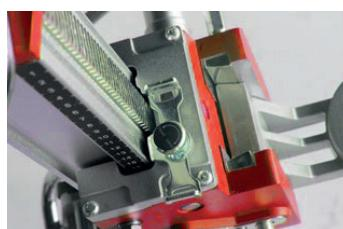
injury or damage to the bit or machine. Slide the carriage lever lock to left to release the carriage, then crank up or down the carriage to the desired position and slide the lever lock to right to lock the carriage in place. Once in position, unlock it and tighten the M6 screw on the lever lock to start operating. Attention! Do not crank up and down the carriage with lever lock in lock position, it will damage both gear rack and the lever lock.
