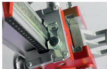
5.1.9 When mounting a 4-bolt rig-mounted type motor, to drill stand COLONNA 250 first use 4 bolts to mount the mounting spacer to the motor. There is a 10x10x100mm key on the mounting plate which can transmit the torque of the motor. Then put the mounting plate with dovetail into the cradle. Tighten the cradle lock bolt until the plate is secured in cradle.
